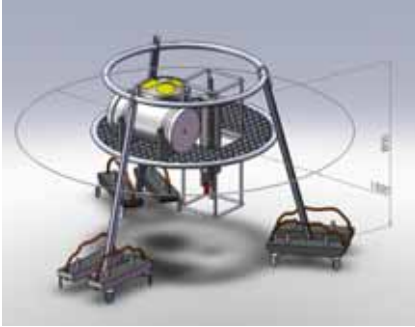
Figure 6: Lander system for the sensors (COSYNA Category I and II)
