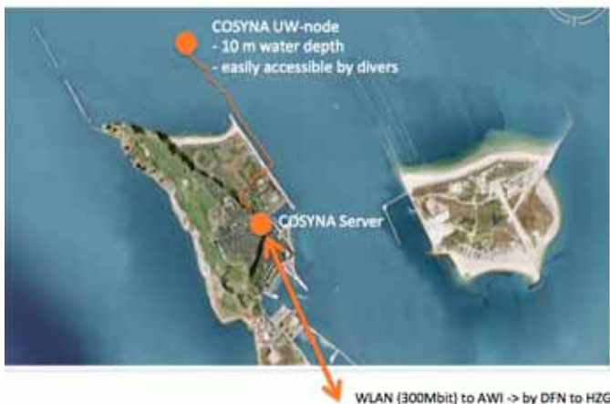
Figure 1: General arrangement of the COSYNA UW-node system off Helgoland
