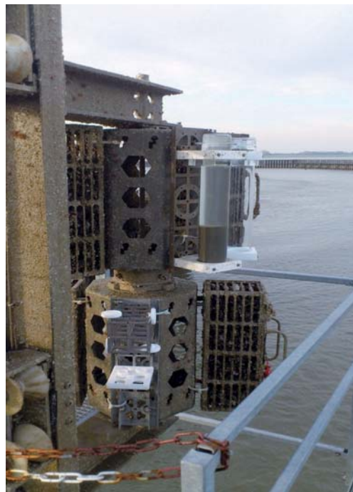
Figure 1: Sampling station at Cuxhaven equipped with integrative (different types of passive and active) sampler
