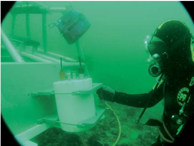
Figure 3: Installing the UW-node system itself and the backup battery pack off Helgoland by the AWI divers.
