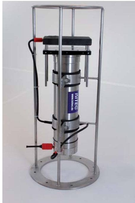
Figure 1: MOKI system with imaging head and attachment frame
