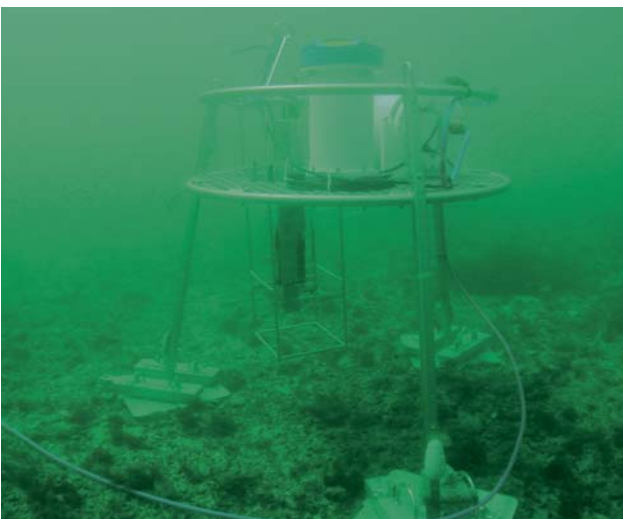
Figure 4: The COSYNA standard lander with a CTD and an ADCP.
