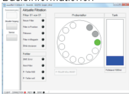
Figure 2: Screen shots of the AUTOFIM software control. The first screen shot (Basisinformationen) provides basic information on the current status of the filtration, including information on the fluid level in the sample reservoir, the number of filters in the storage roundel and the time that passed by since start of the current filtration. The second screenshot (Eingabe Parameter) displays the part of the menu for the definition of the filtration parameter (sample volume, duration of the filtration etc.). Finally, the third screenshot presents the service menu, which allows manual operation of the pumps in the filtration system, e.g. for cleaning of the filtration unit.
