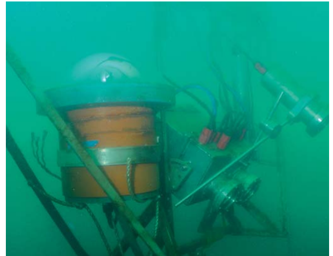
Figure 5: The remote controlled Arctic node system (RemOs1) in NyAlesund (79°N) in 10 m water depth including a CTD, an ADCP and a complex stereo-optical measuring device for fish and jellyfish.
