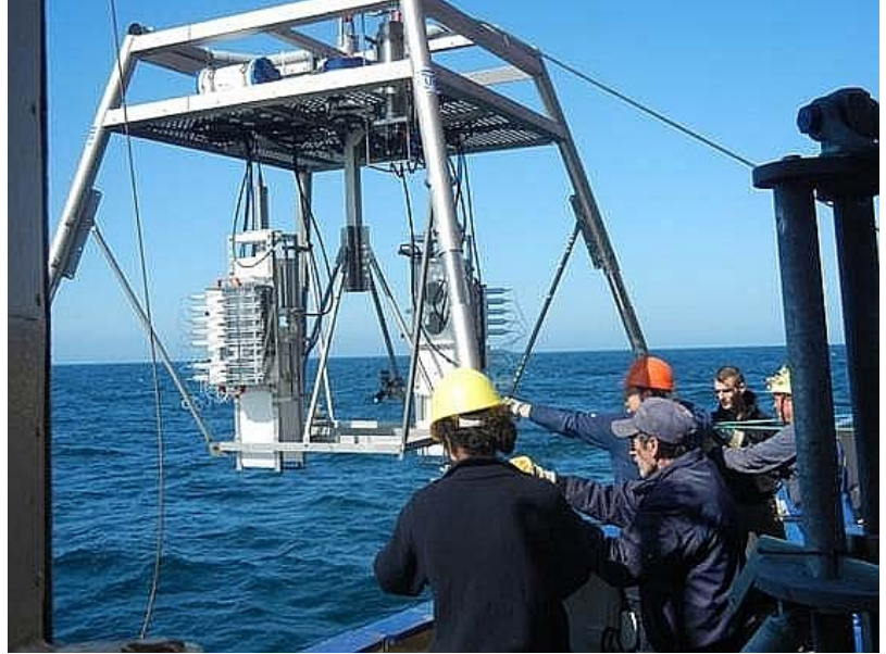
Figure 1: Deployment of the NusObs lander for quantification of benthic fluxes of nutrients, oxygen consumption and transport processes. The lander was deployed for more than 24 hours at the seafloor.
