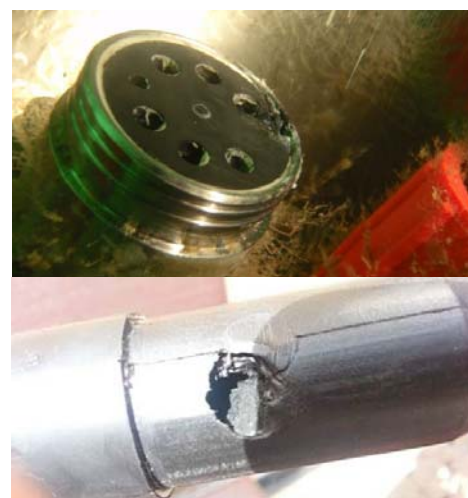
Figure 7: "Burned" plug at the node system at Helgoland.
