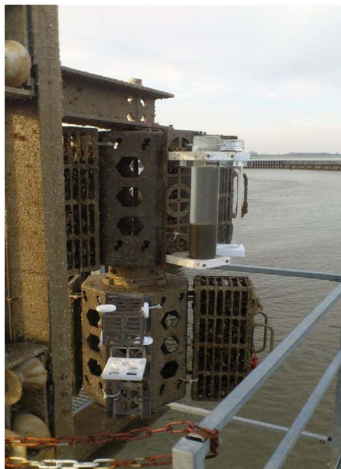
Figure 1: Sampling station at Cuxhaven equipped with integrative (different types of passive and active) samplers, mussel samples
