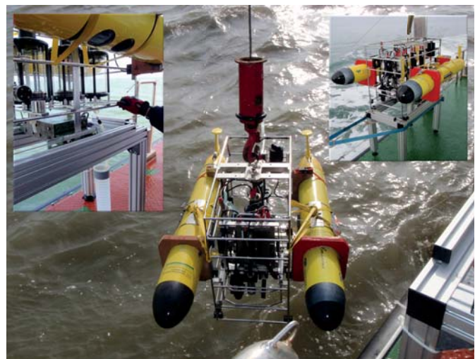
Figure 2: Glider sensor calibration frame, developed at HZG
