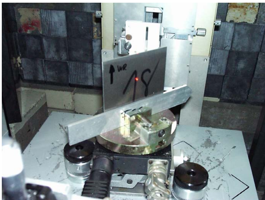
Figure 1: AZ 31 material in measuring position at FSS.
