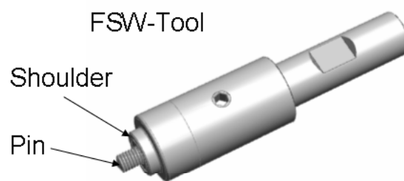
Figure 1. FSW tool pin and shoulder.
