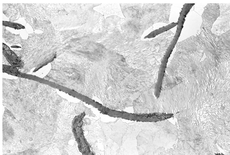
Microstructure GJL, 100% Perlite, 500 x
